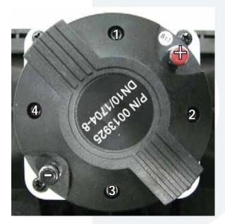
A closeup of the high frequency driver is shown above. Four screws need to be removed from the driver using the 3mm allen wrench.
